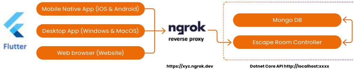
accessing the leaderboard. The game logic is handled in-memory, and when a game is completed, data gets stored in a MongoDB database. This backend solution is locally hosted on one of the Windows laptops and is made accessible externally through an ngrok reverse proxy.
